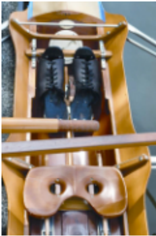
(Laminated seat, leather clogs and "iron back" sculling oars in 1982 Pocock "Standard" racing single)
